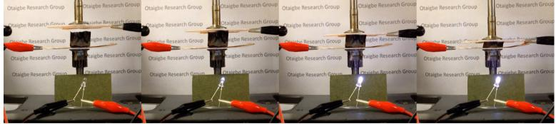
A graphene-polymer aerogel demonstrates the piezoresistive effect, brilliantly lighting up as pressure increases.
