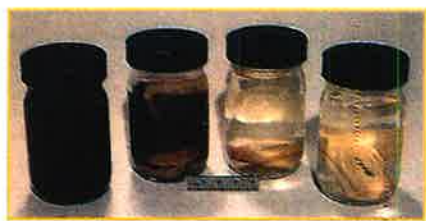
FIGURE 2. A comparison of water resistance of soy-protein polymer and composite: Left to right, unfilled soy-protein polymer, uncoupled composite, coupled composite (method 1), coupled composite (method 2). The coupled and uncoupled composite contained 20 wt% polyphosphate filler, and the materials were immersed in water for 1 year.
