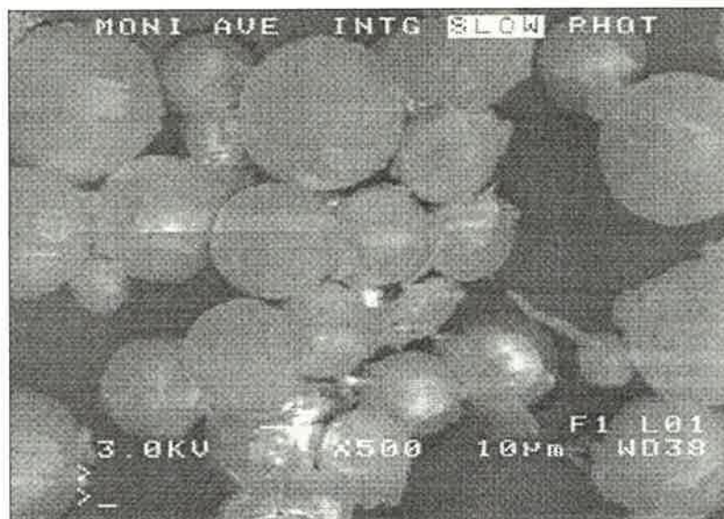
Figure 3 SEM of commercially ground PE-based wax (top), PE520 atomised at pressures of 7.6\text{MNm}^{-2} (above) and 2\text{MNm}^{-2} (below). (The PE520 was atomised at a temperature of 190^\circ\text{C} in both cases)
